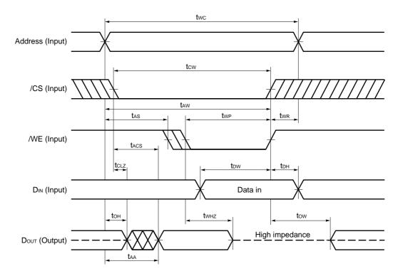
Cautions 1. /CS or /WE should be fixed to high level during address transition.
