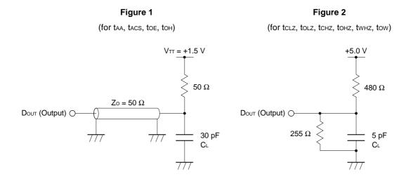
**Remark** CL includes capacitances of the probe and jig, and stray capacitances.
